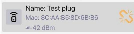
Note: The green checkmark icon means that the Kaidu-plug has been configured and is connected to the network. A yellow broken link icon means the Kaidu-plug is not configured properly or is new.
